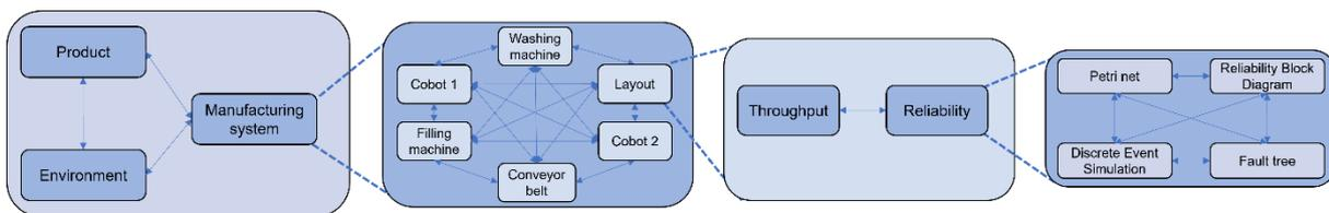
Figure 8: Exemplary design of the different levels of the virtual manufacturing system
