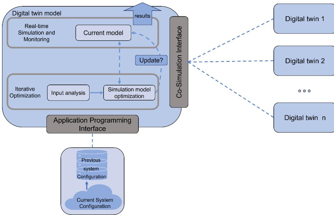
Figure 9: Layout and structure of a digital twin model
