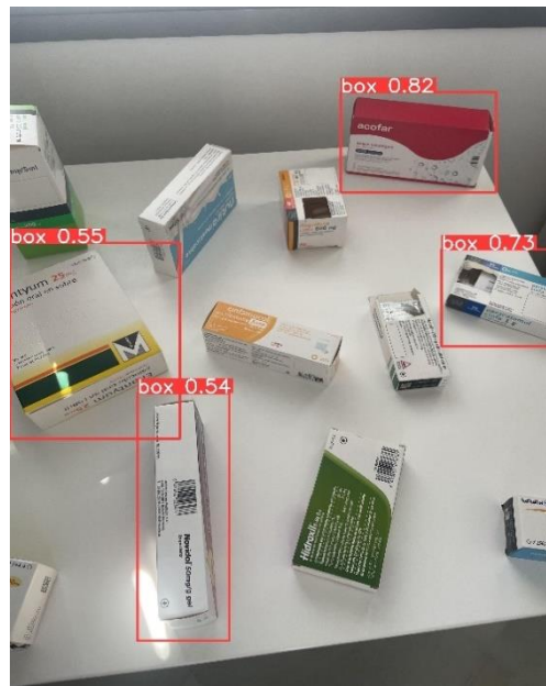
Figure 11. AI-based vision system-trained model results
