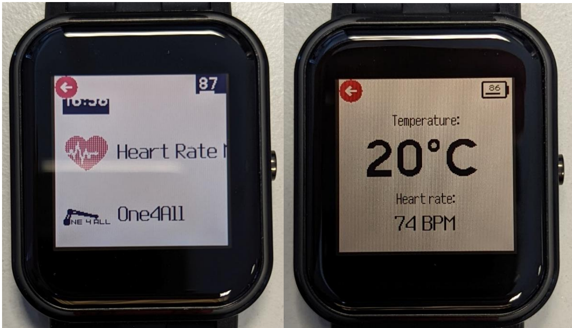
Figure 19 ONE4ALL app in Bangle.JS2 application launcher menu (left) and ONE4ALL app running on Bangle.JS2 (right).
