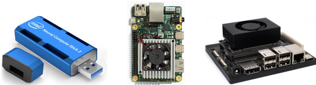
Figure 8 Intel Neural Compute Stick (left), Coral Dev Board (middle), Nvidia Jetson Orin Nano (right)
